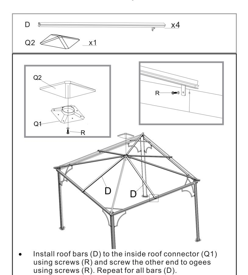
Install the outside roof connector (Q2) to the inside roof
