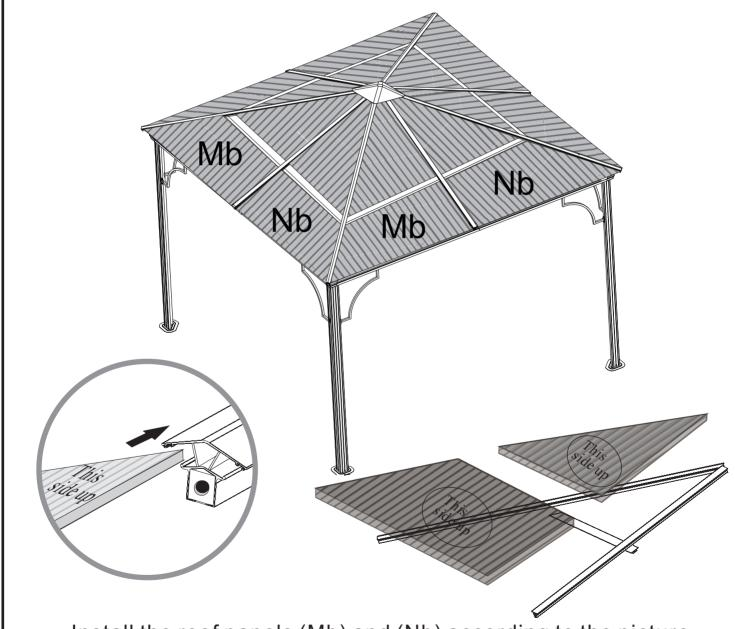
Install the roof panels (Mb) and (Nb) according to the picture.
