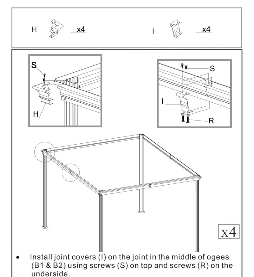
Install corner covers (H) using screws (S).
